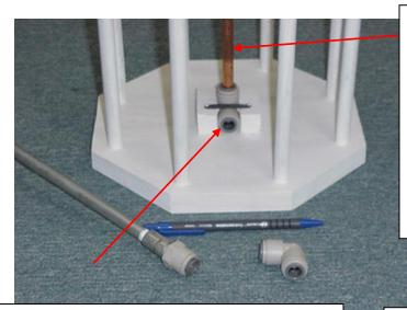
Vertical tube may be any diameter - use a reducer or increaser as necessary to change tube size.
